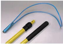
A shepherd's crook should be mounted within 20 feet of the pool and where the people can see it when the pool is open. The pole should be of light, non-electrically conducting material such as fiberglass. It should be non-telescopic, and not less than 12 feet long. It should also have a blunted end with a body hook or shepherd's crook.
